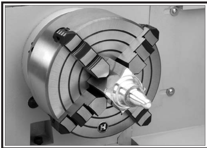
Figure 38. Example photo of non-cylindrical workpiece correctly mounted on the 4-jaw chuck.
